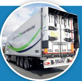
just how big the fuel savings are in real-world situations. Three components were retrofitted to the semitrailer: underfloor panelling (LowFLOW), a trailer bulkhead front spoiler (HighFLOW) and the central component – the RearFLOW rear wing system, pictured – which automatically opens at a speed of 60kph and closes again when the vehicle is driving slowly.
